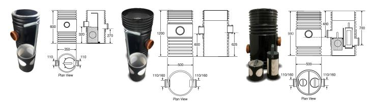
Silt Sentinel 300 series is a small heavy duty silt trap with a removable filter basket under the inlet that will catch the silt in the flow. This product is ideal to locate in the surface drainage runs, between the downpipe and the connecting manhole before the attenuation system. This silt trap will only prevent silt entering the system if the filter bucket and sump is cleaned out regularly but is our most popular selling silt trap.
