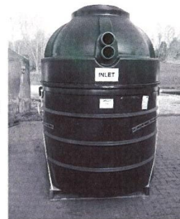
Tank as tested in initial type testing
